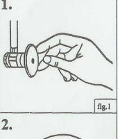
Turn off the water supply to the faucet under sink. Remove existing faucet. Clean area on lavatory surface for installation of new faucet. Make sure drain is closed or blocked to avoid small parts from falling down the drain
